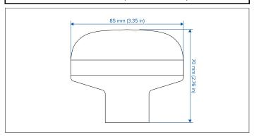
**Important:** If you are replacing a GPS antenna supplied with an older AIS receiver or an AIS700 with an early (low) serial number, please be aware that the mounting diameter (cutout) of the GPS receiver has changed, from Ø44 mm to Ø60 mm.
